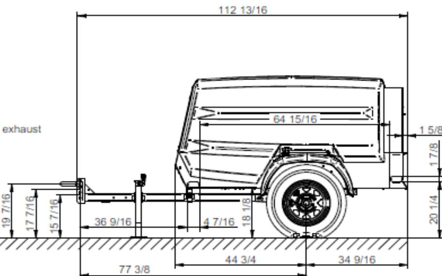
Area covered by the portable compressor (without chassis): 30,35 feet<sup>2</sup>
